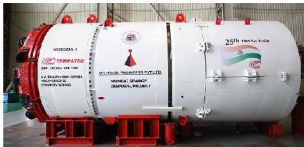
*TERRATEC EPB TBM (TERRATEC)*
