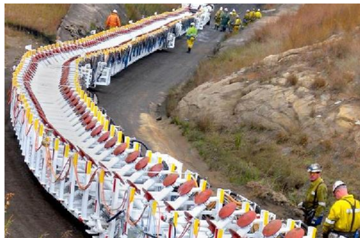
105m langer Flexible Conveyor Train (FCT) von Joy Global
