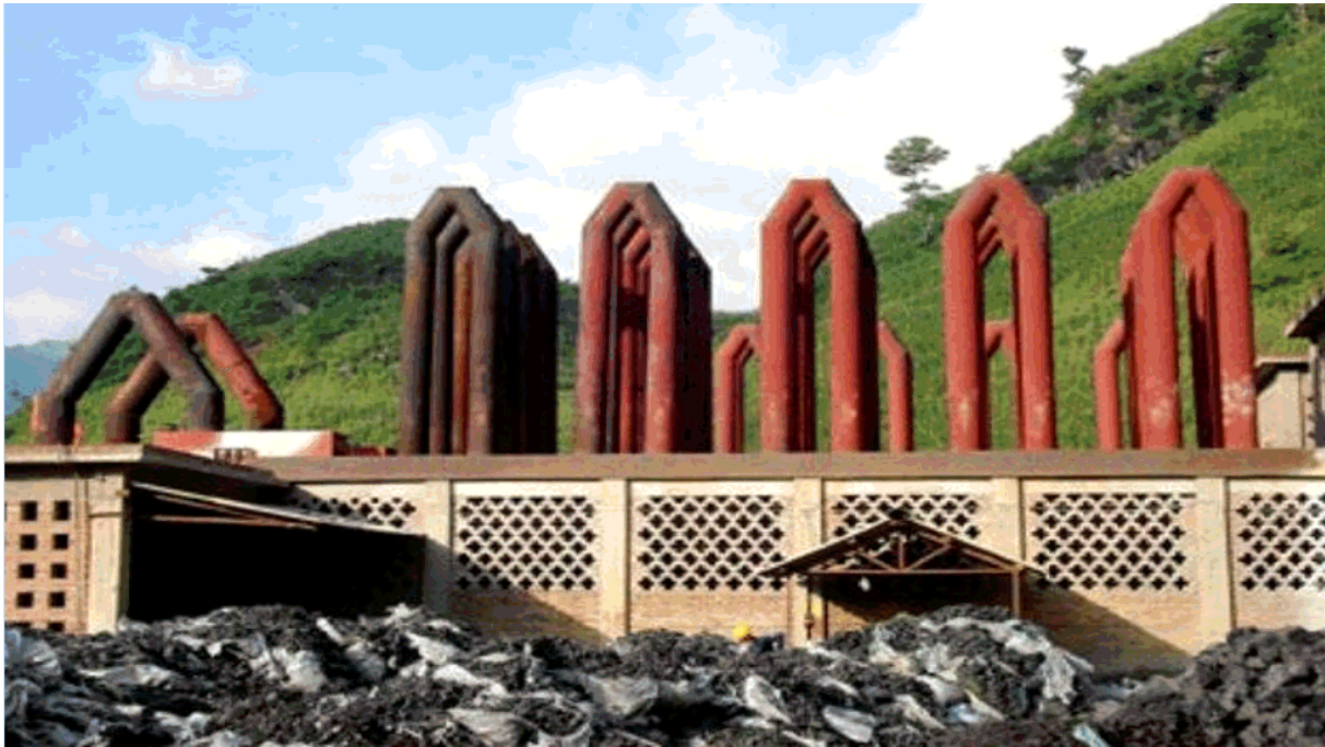
Fig.8 : Antimony Trioxide Condensation Columns at the Mau Due Plant in 2009
